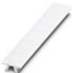
Marker for terminal blocks, Strip, white, labeled, can be labeled with: CMS-P1-PLOTTER, printed horizontally: U, V, W, N, GND, U, V, W, N, GND, mounting type: snap into tall marker groove, for terminal block width: 6.2 mm, lettering field size: 6.15 x 10.5 mm, Number of individual labels: 10
