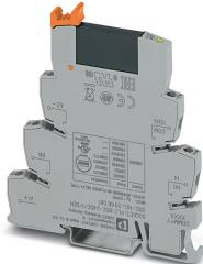
PLC-INTERFACE, consisting of PLC-BSC.../21 basic terminal block with screw connection and plug-in miniature solid-state relay, for mounting on DIN rail NS 35/7,5, 1 N/O contact, input: 24 V DC, output: 24 - 253 V AC/0.75 A
