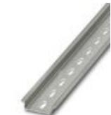
DIN rail perforated, Standard profile, width: 35 mm, height: 7.5 mm, acc. to EN 60715, material: Steel, galvanized, passivated with a thick layer, length: 2000 mm, color: silver
